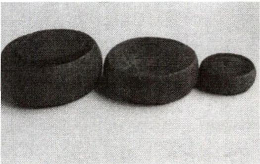
图 1 QB30 钢的 1/3 冷镦样品形貌 Fig. 1 Morphology of 1/3 cold upsetting samples of steel QB30
